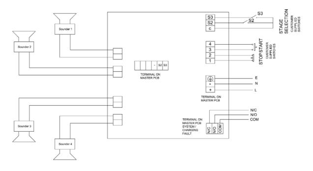
Fig 3: Schematic Circuit Diagram of AC unit with stages S2 and S3 with negative switching
