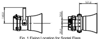
Fig. 1 Fixing Location for Sontel Flare
