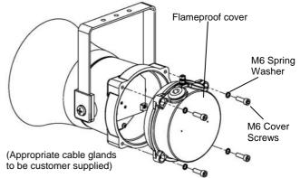
Fig. 2 Accessing the Explosion proof Enclosure.
