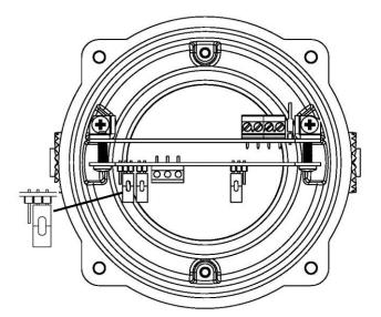
J2 Header Pin - Postion B (pins 2 & 3 linked) places power supply TB Fault resistor & RLY 1-2
