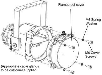
Fig. 2 Accessing the Explosion proof Enclosure.
