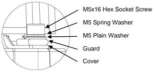
Fig. 13 Cover and Guard Fixtures
