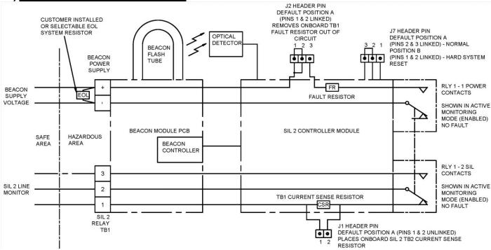
Fig 4 - The SIL 2 Module monitors the Beacon and interfaces to the customer plant.
