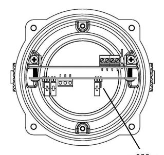
J7 Header Pin - Postion A, Factory default position (pins 2 & 3 linked) set to normal operation.
