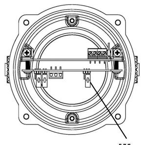
J7 Header Pin - Postion B (pins 2 & 3 linked) set for hard reset.
