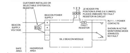
Figure 7 - Schematic of SIL 2 system wiring for fault detection in standby mode only - 2 wire installation
