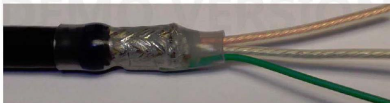
FIGURE 5 DATA CABLE (PL10836) WITH SOLDER SLEEVE (PL10836-S)
