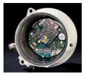
Light Guard GSM GSM unit and antenna integrated in the lantern for remote monitoring and control.
