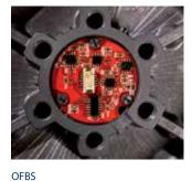
The Optical Feedback System (OFBS) enables built-in monitoring of LED degradation over time.
