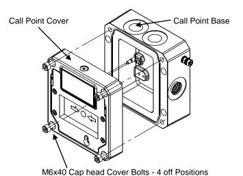
Fig. 2 Accessing the Explosion proof Enclosure.
