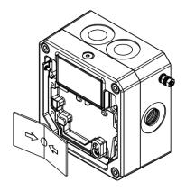
To fit the new glass element rotate the top cam clockwise by an angle of 50° (use a 6mm Allen key) this will than allow the glass to fit back into the pocket it sits in, resting on the pivot point and test cam, release the top cam to rest on the top of the glass element.
