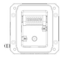
Fig. 4 DIN Rail in Base
