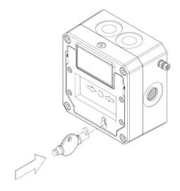
The test key is inserted in the test cam and rotated clockwise by an angle of 90° the glass element will visibly drop down in the viewable window.
