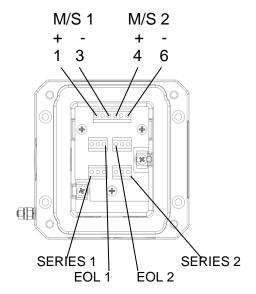
Fig. 5 PCB Terminal Block in Base
