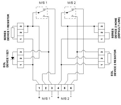
5A - Circuit as shown in Unoperated condition Terminals +(1) & -(3) M/S 1 and +(4) & -(6) M/S 2 open Terminals +(1) & (2) M/S 1 and +(4) & (5) M/S 2 closed
