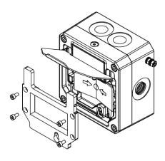
Once the cover is removed the broken glass will be free to be removed, clean out any other fragments of glass carefully.
