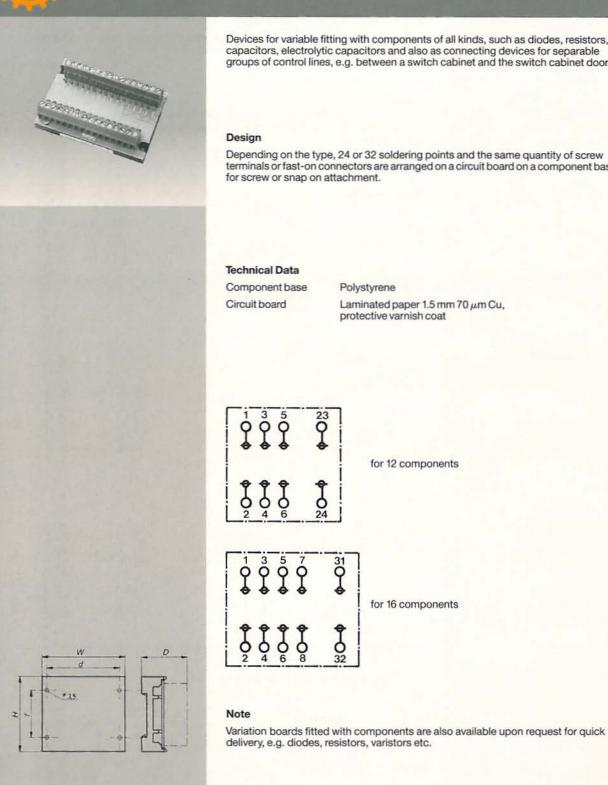
Devices for variable fitting with components of all kinds, such as diodes, resistors, capacitors, electrolytic capacitors and also as connecting devices for separable groups of control lines, e.g. between a switch cabinet and the switch cabinet door.
