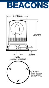
The R401/400 Din Base Series uses a parabolic reflector which, driven by an electric motor, revolves around a continuously illuminated lamp on the vertical axis of the beacon creating a powerful beam of light travelling through 360
