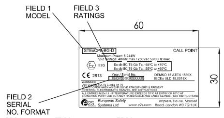
FIELD 1 FIELD 2 FIELD 3 MODEL SERIAL NO. FORMAT RATINGS
