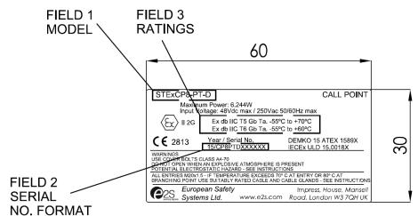
FIELD 1 FIELD 2 FIELD 3 SERIAL NO. FORMAT **RATINGS** MODEL
