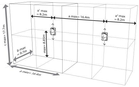
Signaling ranges of the PYRA flashing light PY X-M-10, 24 V AC/DC, red lens, using the example of wall mounting
