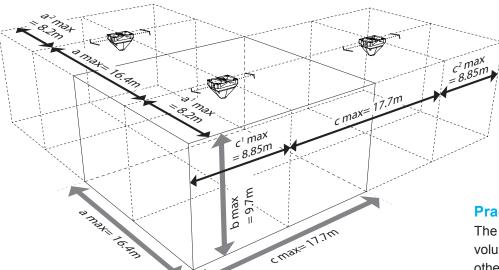
Signaling ranges of the PYRA flashing light PY X-M-10, 24 V AC/DC, red lens, using the example of **ceiling mounting**
