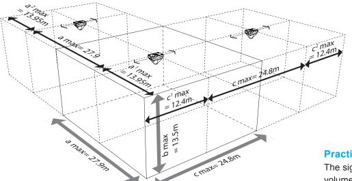
Signaling ranges of the PYRA flashing light PY X-M-10, 24 V AC/DC, clear lens, using the example of ceiling mounting
