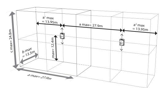
Signaling ranges of the PYRA flashing light PY X-M-10, 24 V AC/DC, clear lens, using the example of wall mounting
