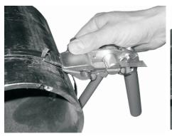
1. With the Bantam Tool in the Pistol Grip Position, Place the band in the tool with sufficient band in the winding mandrel.
