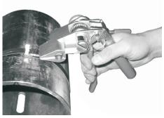
2. With ratcheting action, tension the band until clamp is tight. If necessary, band may be repositioned be releasing tension with levers.
