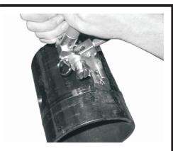
3. Roll tool over as far as tool will go, and push forward cutter handle. Remove tool and tap or hammer down ears of clip to complete clamp. Remove excess material from winding mandrel.
