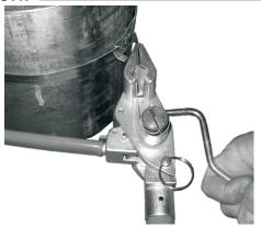
3. Roll tool over as far as tool will go, and push forward cutter handle. Remove tool and tap or hammer down ears of clip to complete clamp.
