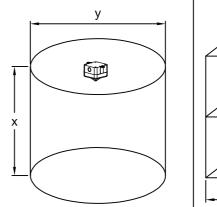
Category C-x-y (Ceiling mounted): Ceiling mounted, where x is the maximum ceiling height and y the diameter of the cylindrical volume covered by the VAD.
