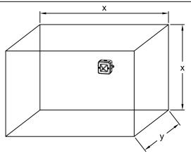
Category O-x-y (Open class): Centrally wall mounted, where x is the max height and width of the wall area covered by the device and y is the max depth of the volume covered by the VAD or ceiling mounted where x is the max width and length of the floor area covered of the VAD and y is the max ceiling height.
