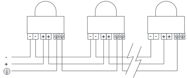
Fig. 5 D2xB1X05/D2xB1X10 DC Simplified Block Diagram
