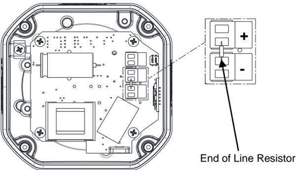
Fig. 8b End of Line Resistor Placement (D2xB1DC024)
