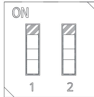
Fig. 7 DIP Switch setting '00'
