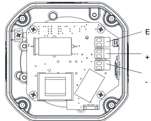
Fig. 6b D2xB1X05/D2xB1X10 24 VDC Terminals
