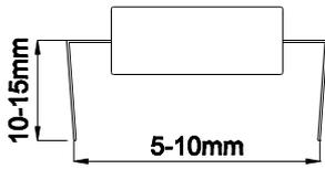
Fig. 7 End of Line Resistor Forming
