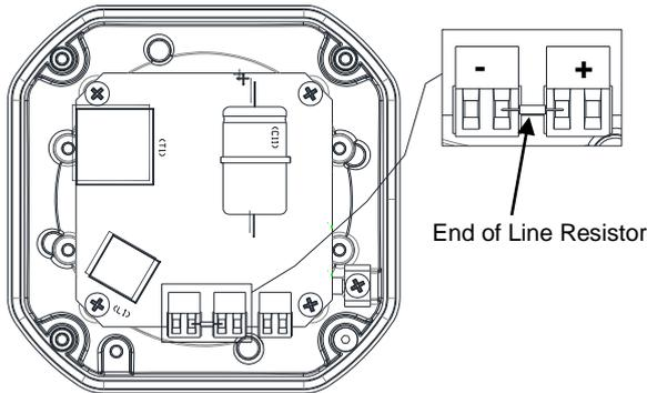
Fig. 8a End of Line Resistor Placement (D2xB1DC048)
