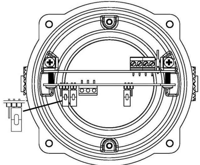
J2 Header Pin - Position B (pins 2 & 3 linked) places power supply TB Fault resistor & RLY 1-2
