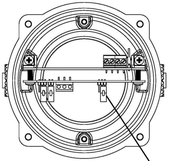
J7 Header Pin - Position B (pins 2 & 3 linked) set for hard reset.
