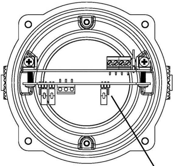
J7 Header Pin - Position A, Factory default position (pins 2 & 3 linked) set to normal operation.
