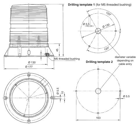
Two different drilling templates are available for fixing the light (direct mounting). M5 x 8 threaded bushes are set into the base of the light for fixing according to drilling template 1. Drilling template 2 allows the light to be fixed using 4 through bolts or similar from above.
