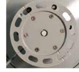
The bottom plate of the LED 350 supports installation on structure using 3 x M12 bolts or 4 x M12 bolts on a 200 mm radius. The mounting holes are galvanic isolated with plastic isolators. PTFE breathing vent for pressure release.
