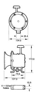
The ES is a manually operated hooter producing the unique 'Klaxon' sound for applications where a power supply is unavailable. Typical
