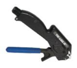
Applies 6.35mm wide smooth ID Tie-Lok® ties used in cable bundling and identification tagging. Locks tie with the patented Tie-Lok® and cuts off excess band flush with top of buckle so the completed lock is smooth and not sharp.
