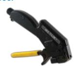
Quickly, easily and consistently applies any size Multi-Lok ties. Simply adjust the Multi-Lok tool for the desired tension, side load the tie into the tool and squeeze the handle. When the proper tension is reached, the Multi-Lok tool automatically cuts the tail off close to the buckle.
