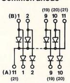
The numbers in brackets refer to diode devices with 40 diodes.
