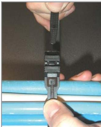
Insert the tip of the tie and tighten a short segment.
