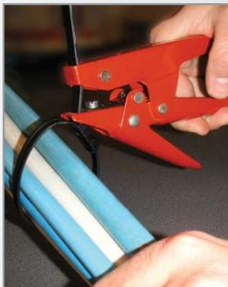
Use the tool for tightening the tie around the cables.
