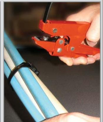
Cut the exceeding part of the tie with the tool, leaving at least one centimeter of safety length.
