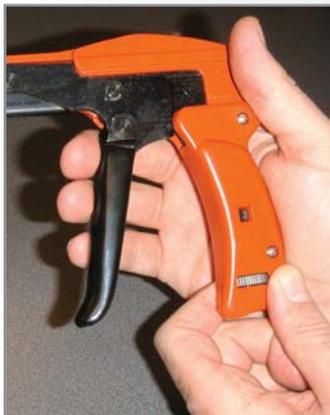
Set the max tension of the tool depending on the size of the tie.
