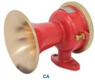
These air horns are for general signaling services. They generate sound by means of a vibrating diaphragm that modulates the flow of compressed air into a resonating projector. All horn shapes are mathematically calculated to amplify sound while closely retaining its fundamental frequency and natural harmonics. All horn frequencies are designed to give balance to any combination of horn tones.
