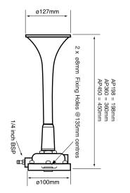
The AP Series of air horns are suitable for general purpose signalling where high output is required such as foundries, steelworks and petrochemical plants. Operated from a
