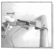
Push axle handle so the band can be placed in slots of tool. Push nose of tool against the buckle.
