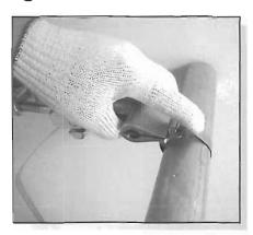
Place finger on buckle bridge and apply tension by turning handle.
