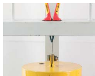
50 KG weight test on insulated sleeve
