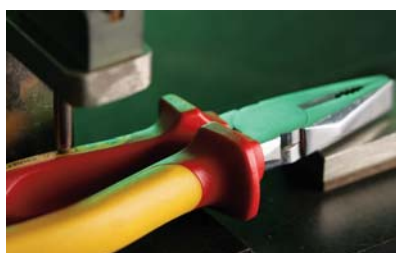
Tolerance test after hot and cold shock test
