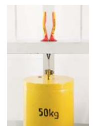
50 KG weight test on insulated sleeve
