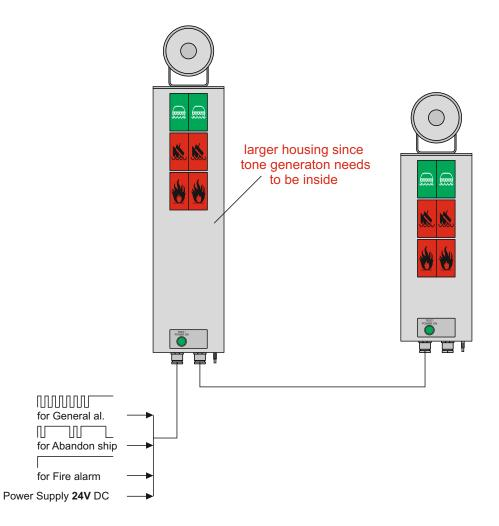
Input contact for General alarm should follow general alarm sequence waveform (7 short and 1 long).
